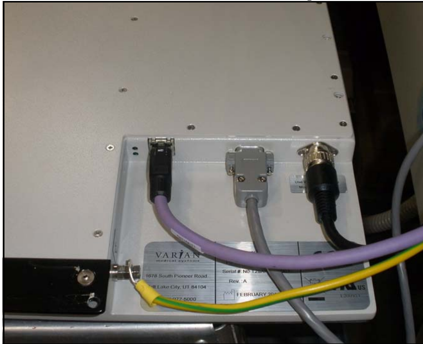
Figure Addendum D-26. Receptor Cable Connections
